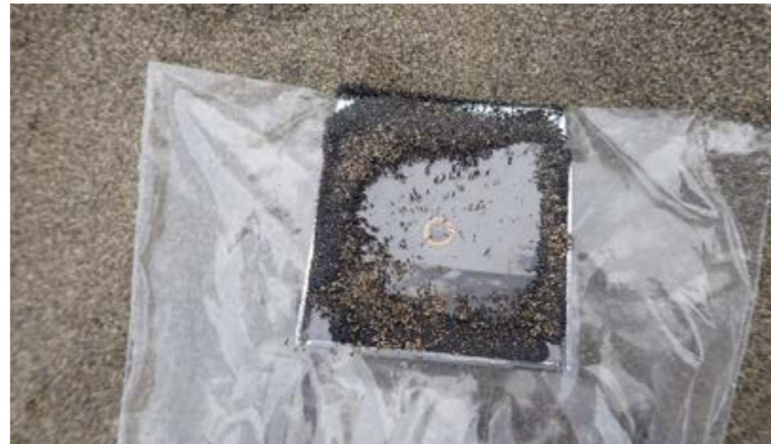
▲用塑膠袋包住磁鐵吸附磁鐵礦砂
